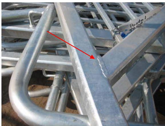
Galvanized guardrails – welds rejected, typical
